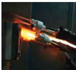
Thermal spray cooling technology uses -195^{\circ}\text{C} nitrogen
